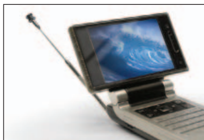
▲ Fig. 1 Initial mobile-TV handsets required use of an external whip antenna.
