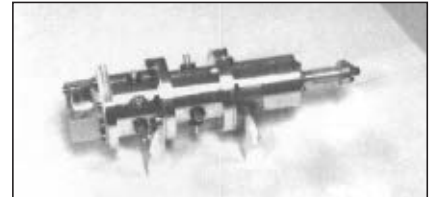
▲ Fig. 6 Five-element dual-mode filter prototype.
